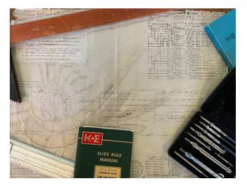
Above is a montage of drawing and calculating instruments, lying on our 1959 drawing of the 19 element CANDU fuel bundle for 3-inch pressure tubes (i.e., NPD and Douglas Point). The drawing (pencil on vellum) is stamped by the late Les Haywood, PEng, a senior reactor designer/manager at Canadian General Electric in Peterborough and later AECL; the museum has several items linked to Les, including a beautiful coffee table made for his retirement.
