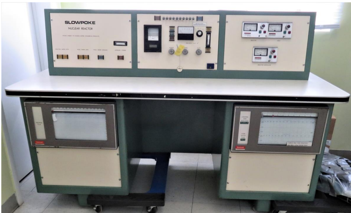
Figure 2: The console from the University of Alberta SLOWPOKE reactor.
